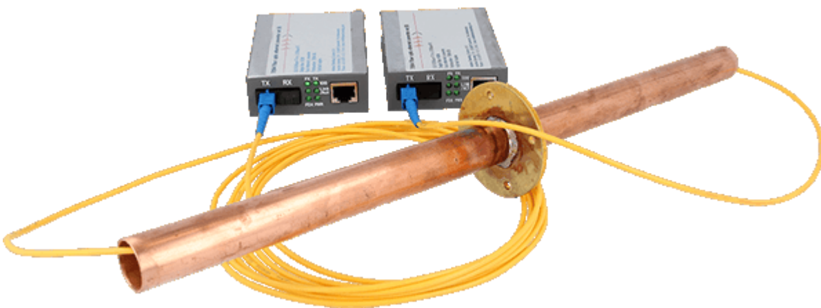
Feedthrough set for shielded rooms and Faraday cages. The unit outside the Faraday cage is connected with the unit inside the Faraday cage through a waveguide an optical fiber.
