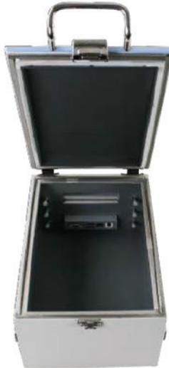
Medium shielded box to block wireless communication during testing and measurements working size 230(W)*320(D)*160(H)
