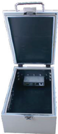
Compact shielded box to block wireless communication during testing and measurements working size 210(W)*354(D)*120(H)
