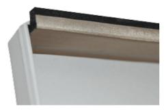
In the picture above you can see how the gasket can be mounted on the inside of the lid. The L-shaped EMI / RFIshielding gasket can be mounted with a self-adhesive that can optionally be conductive. When the lid is closed, the electrical contact is shielded from water and dust.
