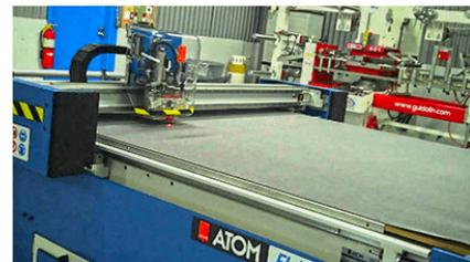
Conductive felt can be cut into any shape by our CNC cutting machine.
