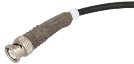
*4955 series Cable connector shield used to shield a plastic connector. The Cable connector shields is connected to the shield beneath the black plastic cable jacket with a 4703 Amucor tape.*
